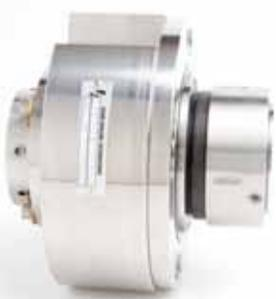
**Type C / Arrangement 1 single seal** has a high temperature stationary metal bellows element as the standard configuration. Rotating bellows are optional and must be called out on the data sheet. In addition to the porting and bushing options for Type A/B seals, the Type C seal can be supplied with a steam purge bushing for more efficient steam quench in coking applications.
