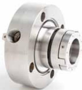
**Type A / Arrangement 1 single seal** has a rotating flexible element as the standard configuration. Stationary flexible element is optional and must be called out on the data sheet. Standard flush is single point, and standard restriction bushing is fixed design. Optional multi-port flush as well as floating or segmented bushings are supplied based on application requirements. A pumping ring is also available when seal is designed for API Plan 23 operation.
