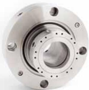
**Type B / Arrangement 1 single seal** has a low temperature rotating metal bellows element as the standard configuration. Stationary metal bellows is available as an option and must be called out on the data sheet. The porting and bushing standards and options are the same as the Type A seal.
